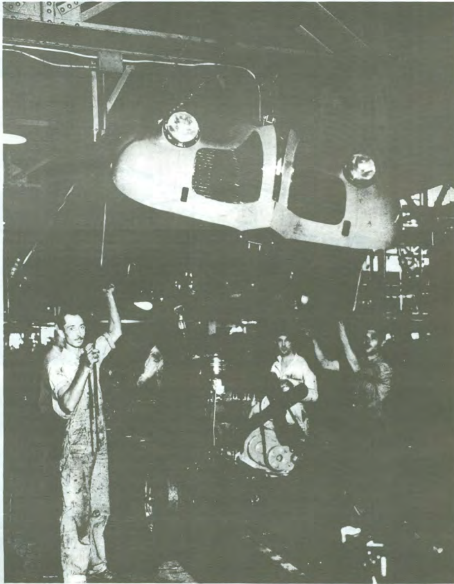
At this stage, when the front fender and radiator shell unit are dropped into place on the chassis, a layman watching a car grow in the Southern California Division of General Motors knows whether it will be a Buick, Oldsmobile or Pontiac. Yes, this one is a 1940 Pontiac, almost ready to receive its body
